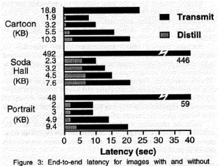
Figure 3: End-to-end latency for images with and without distillation. Each group of bars represents one image with 5 levels of distillation; the top bar represents no distillation at all. The y-axis number is the distilled size in kilobytes (so the top bar gives the original size). Note that two of the undistilled images are off the scale; the Soda Hall image is off by an order of magnitude.
